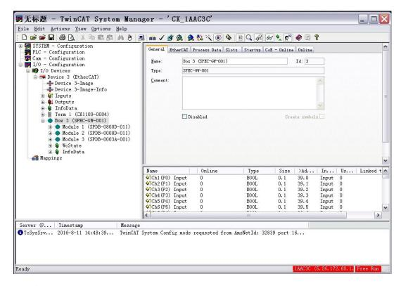
3) In order to configure specific modules and send them to PLC to ensure the normal use of subsequent power-ups, it is necessary to check the "Download Slot Configuration" option in the Slots label.
