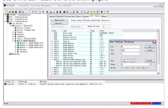
5) After all the settings are completed, click on the "Reload I/O Devices" button and download all the information to the PLC. At this time, the module should be in the connection state and the MOD indicator light should be in the evergreen state.
