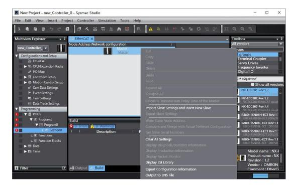
5) Right-click on the PLC icon and select the item "Configuration and Merge with Physical Network" to see the following interface. You can see the FEEC module appears at A, then click on B, until the FEEC module icon appears under the PLC in the list on the left.
